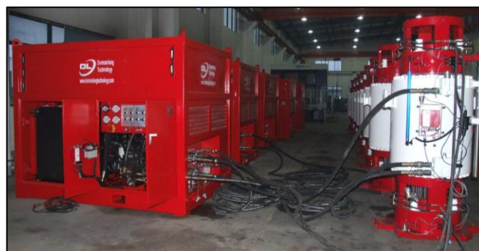
Typical diesel powered hydraulic power units and DL-S588 strand jacks
