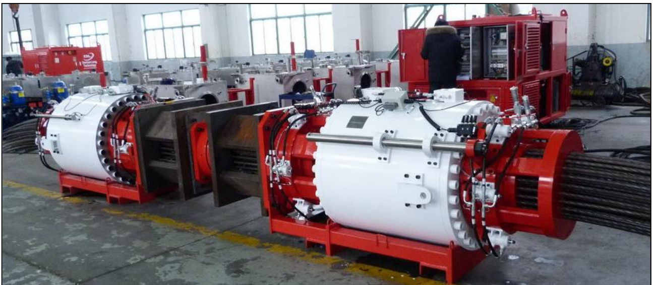
2No. DL-S836 strand jacks during 125% load testing in factory (with transport frames)
